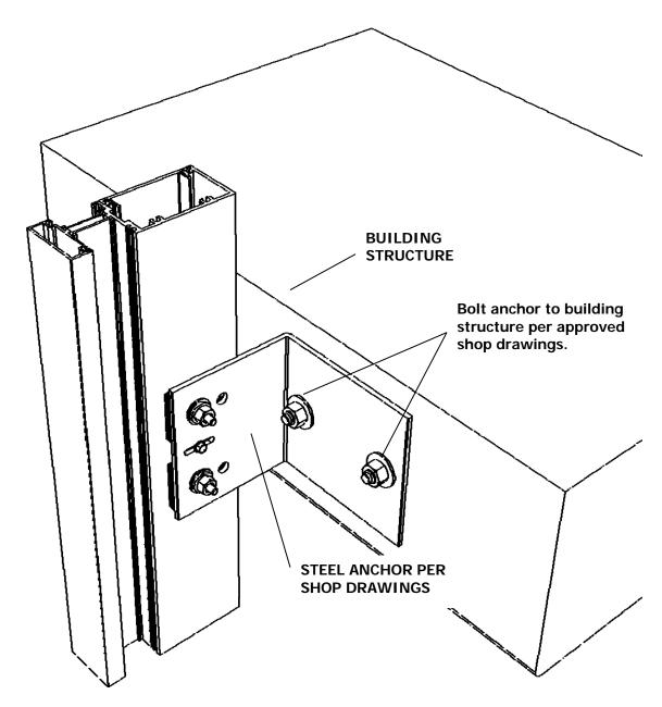
NOTE: The elevation of the structure must be within the adjustment limits of the anchoring system. See approved shop drawings for limitations.
