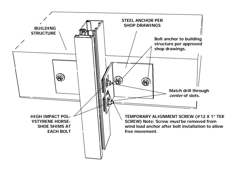
**BOLTED WIND LOAD ANCHORS**
