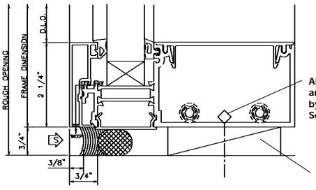
Note: It is up to the responsible engineer to determine the structural adequacy and type of anchorage method to be used for a given substrate, applied loads, and building movements. The S-5500 has different anchorage options available to meet these conditions.
