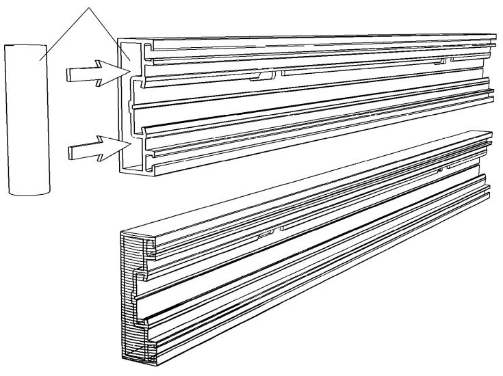
NOTE: Exterior pressure covers to be cut D.L.O. minus 1/8" at typical lites and D.L.O. minus 3/16" for lites on the deep pocket side of the expansion mullions.
