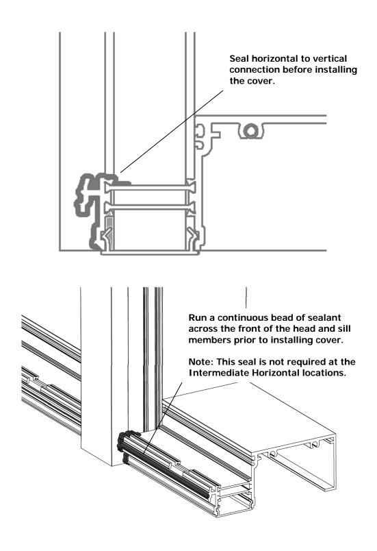
STEP #2 (Option A) APPLY HORIZONTAL 2 PIECE PRESSURE PLATE AND COVERS
