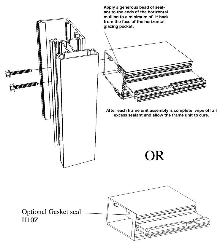
Install gasket to each end of horizontal before attaching to vertical. Trim excess gasket material after assembly.
