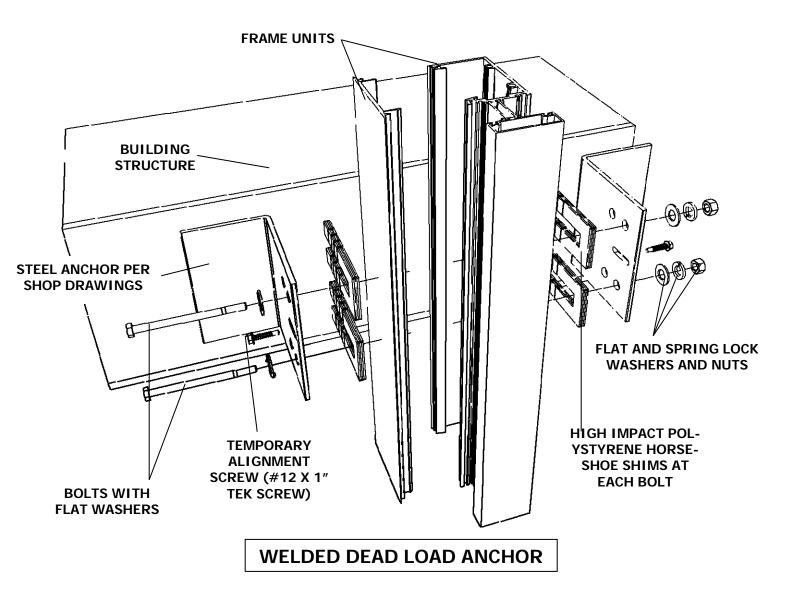
NOTE: When welding, protect installed metal and glass from weld splatter.
