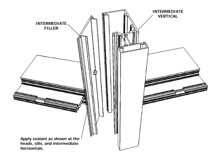
Note: Care should be taken when handling the frames to avoid damaging the edges of the fillers. A block of wood and "C" clamps should be used to aid in snapping the filler to the mullions.
