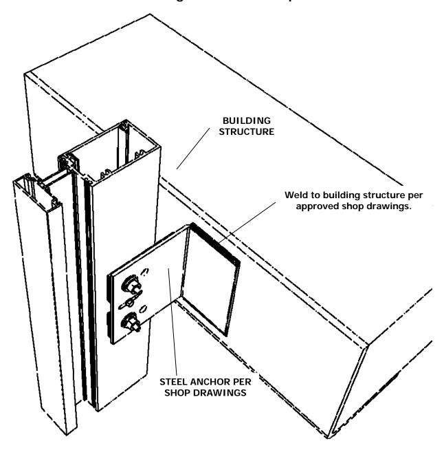
NOTE: The elevation of the structure must be within the adjustment limits of the anchoring system. See approved shop drawings for limitations.
