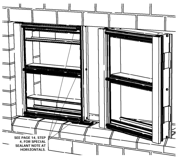
NOTE: On long runs, check overall frame dimensions at every fifth opening to avoid dimensional build-up. The commercial cut length tolerance is +/- 1/16". It is critical to check every fifth unit for location relative to established benchmarks.
